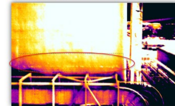
Figure 27: Top and Below, hotter white areas indicate material voids and loose material. White spot following straight lines typically indicate a joint that is not effectively repaired
